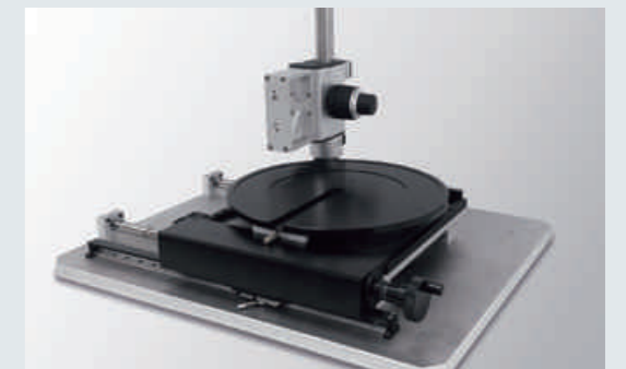
A stand that allows you to observe a disk-shaped object from the edge to the center while rotating it. Compatible with 12 inch wafers.
